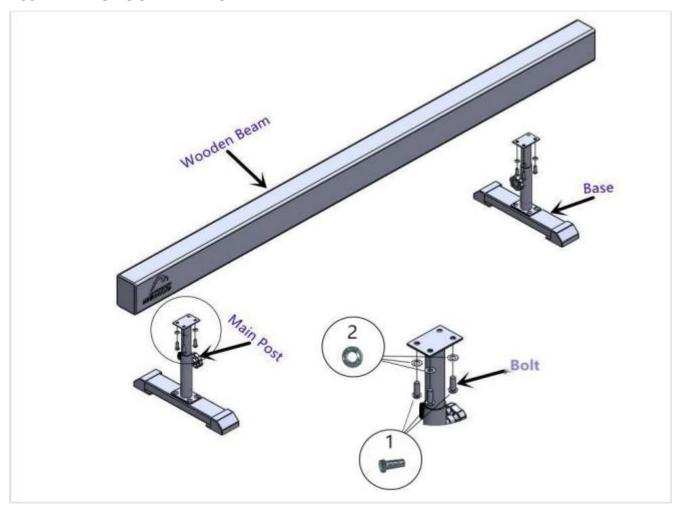
Please put Main Post B into Main Post A before assembling, providing you with 2 Main Posts, as shown in the picture.
